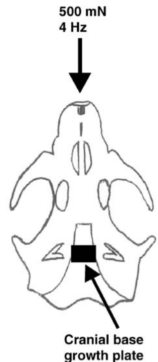
Fig. 1 Representation of the rat cranial base growth plate (CBGP) showing the application of exogenous mechanical forces (cf. Almubarak et al. 2005; Collins et al. 2005). The direction of mechanical forces applied to the rat maxilla at 500 mN and 4 Hz for 20 min/day over two consecutive days is indicated ( downward pointing arrow ). The applied exogenous forces were transmitted as mechanical strain to bone adjacent to the CBGP (Oberheim and Mao 2002)
