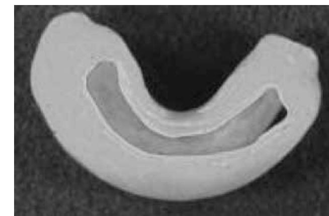
Figure 4 Top view of tray is shown. Wax from inside of Triad material was removed and will be replaced with Cerrobend metal through the opening on the top. This opening will then be closed with more triad material to seal the metal inside.
